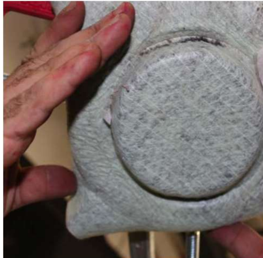
Bottom view, some tears in the external fabric, but no leakage
