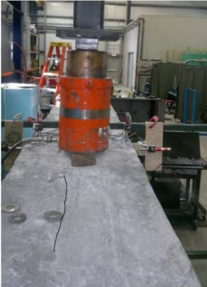
Flexure Failure in the Middle Concrete Unit
