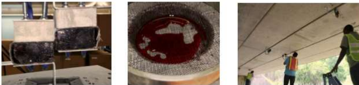
Fig. 2 Differential Deflection Test (Left); Leakage Test (Middle); and Deflection Measurements (Right)
